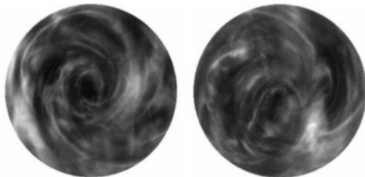
**Figure 3** Two snapshots of the flow at  $Wi = 13$ ,  $Re = 0.7$ . The flow under the black upper plate is visualized by seeding the fluid with light reflecting flakes (1% of the Kalliroscope liquid). The fluid is illuminated by ambient light. Although the pattern is quite irregular, structures that appear tend to have spiral-like forms. The dark spot in the middle corresponds to the centre of a big persistent toroidal vortex that has dimensions of the whole set-up.
